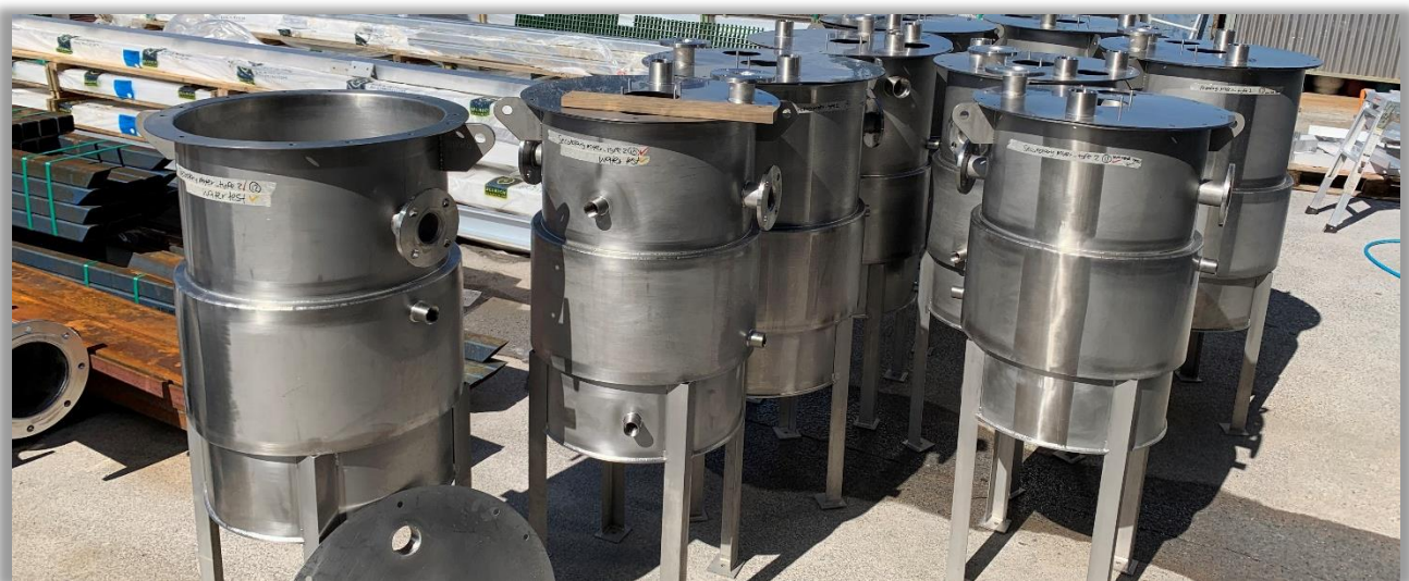
Completed SX mixer tanks ready for shipping
