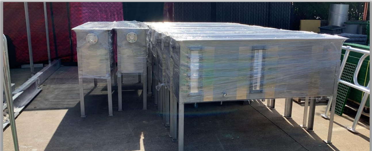
Completed Solvent Extraction (SX) settler tanks ready for shipping
