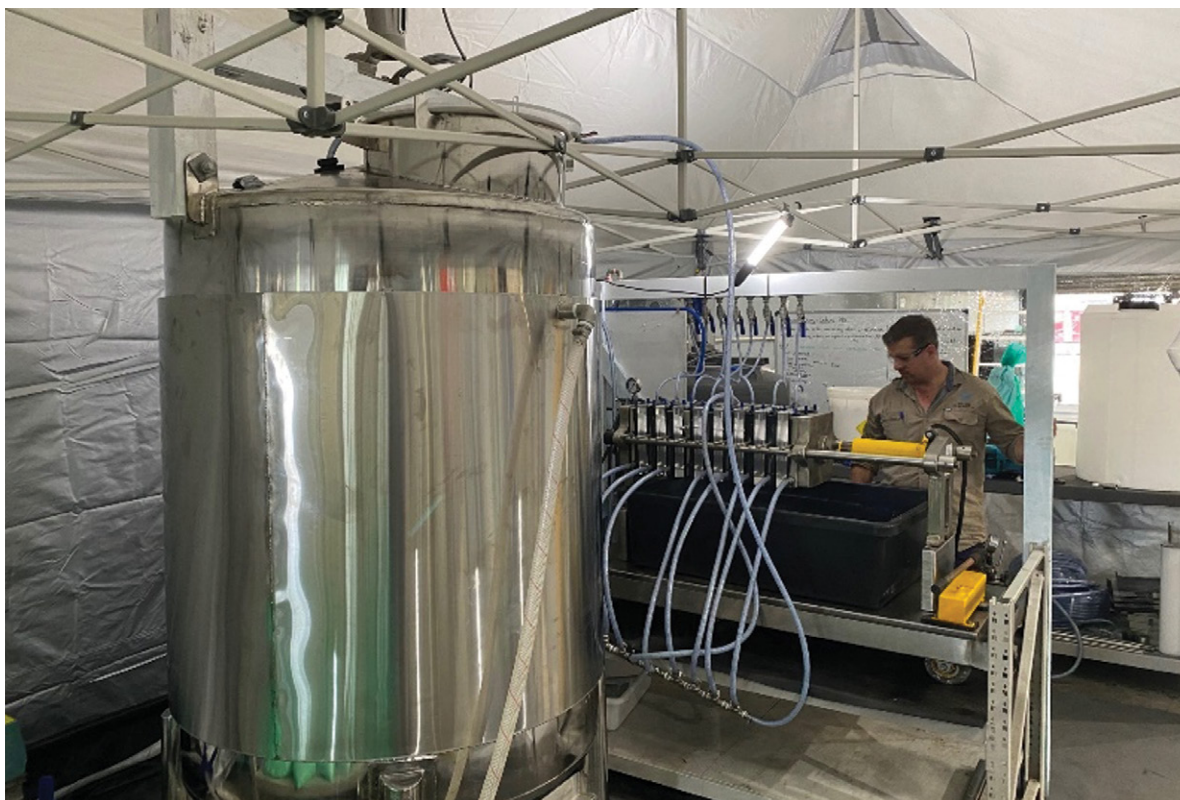
Demonstration scale pre-cursor circuit generated 99.998% purity HPA
