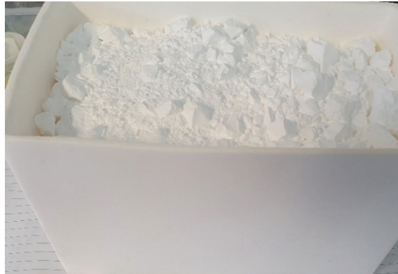
A batch of HPA pre-cursor ready for calcination
