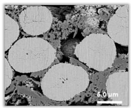
Al doped high nickel (NCMA811) cathodes after 1,000 cycles Source: Kim et al, ACS Energy 2019
