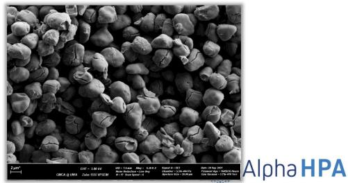
HPA coated Li-B anodes for EU anode OEM
