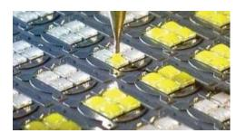
Addition of YAG phosphors to LED lighting circuits
