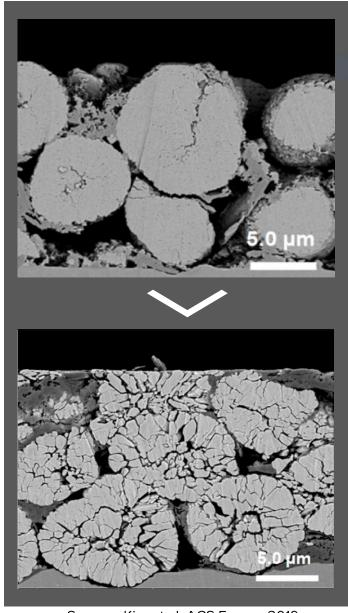
Breakdown of high nickel (NCM811) cathodes after 1,000 cycles
