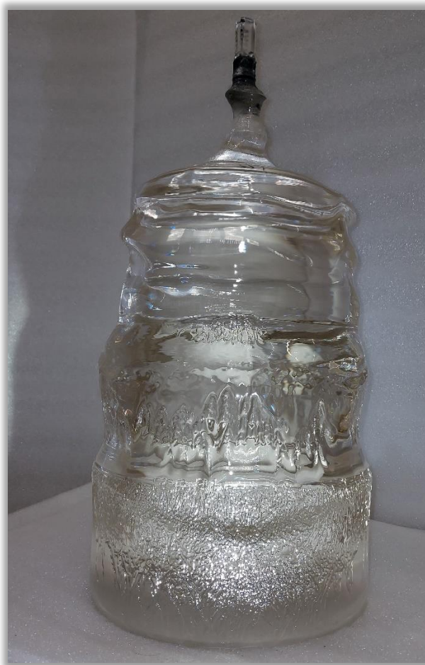
~90kg single crystal sapphire glass boule grown by ALOX using Alpha feedstock
