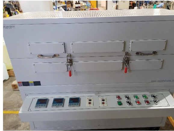
Large capacity, rotary calciner on-site at the Pilot Plant
