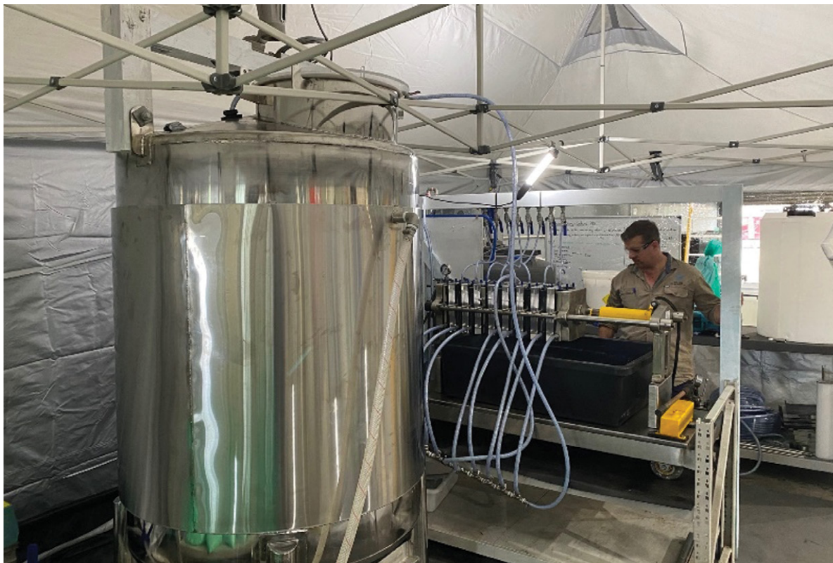
Demonstration scale pre-cursor circuit generated 99.998% purity HPA
