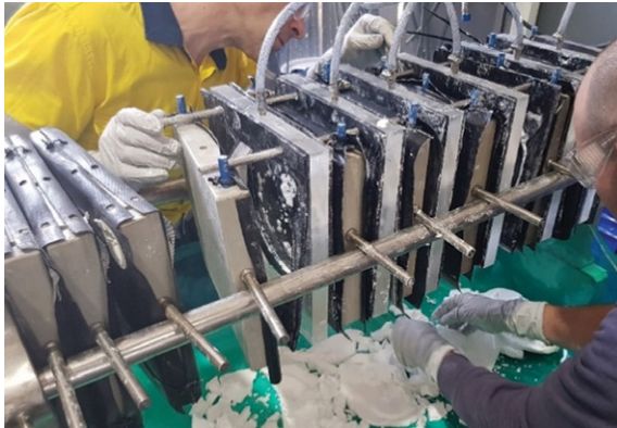
Removal of HPA pre-cursor from the filter
