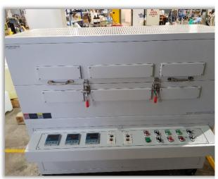
Large capacity, rotary calciner on-site at the Pilot Plant
