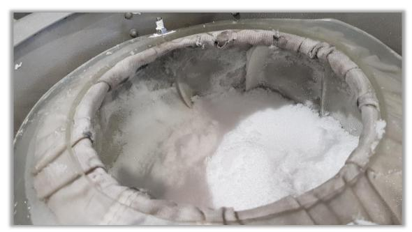
A centrifuge batch of high-purity pre-cursor product (approx. 2kg) produced at Alpha HPA's demonstration facility
