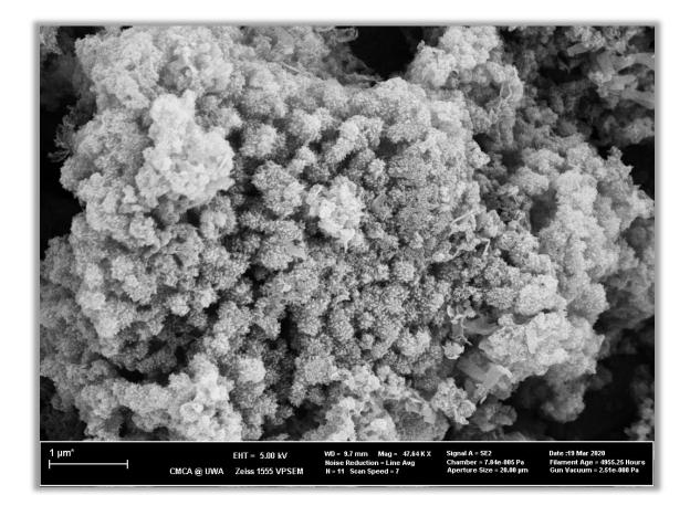
Appendix 2: Gamma Alumina under SEM (Scanning Electron Microscope)
