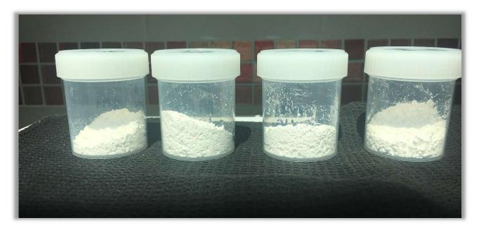
High Purity Alumina produced from the second SX mini-rig run
