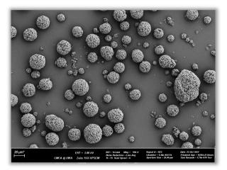
SEM image of Alpha's spherical gamma alumina.
